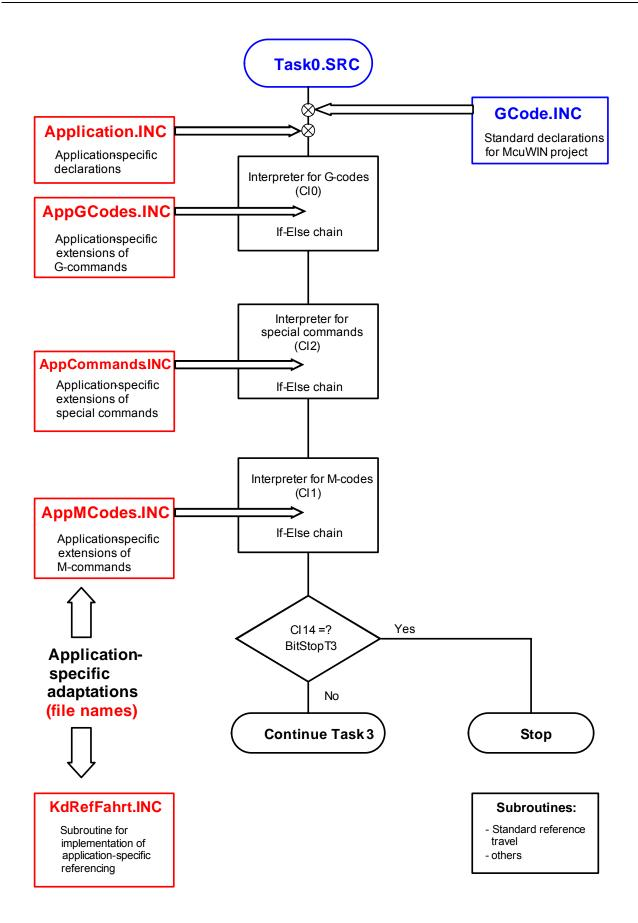
The blocks shown in red on the left-hand side of the flowcharts are the application-specific extensions. These are not replaced in case of updates.
