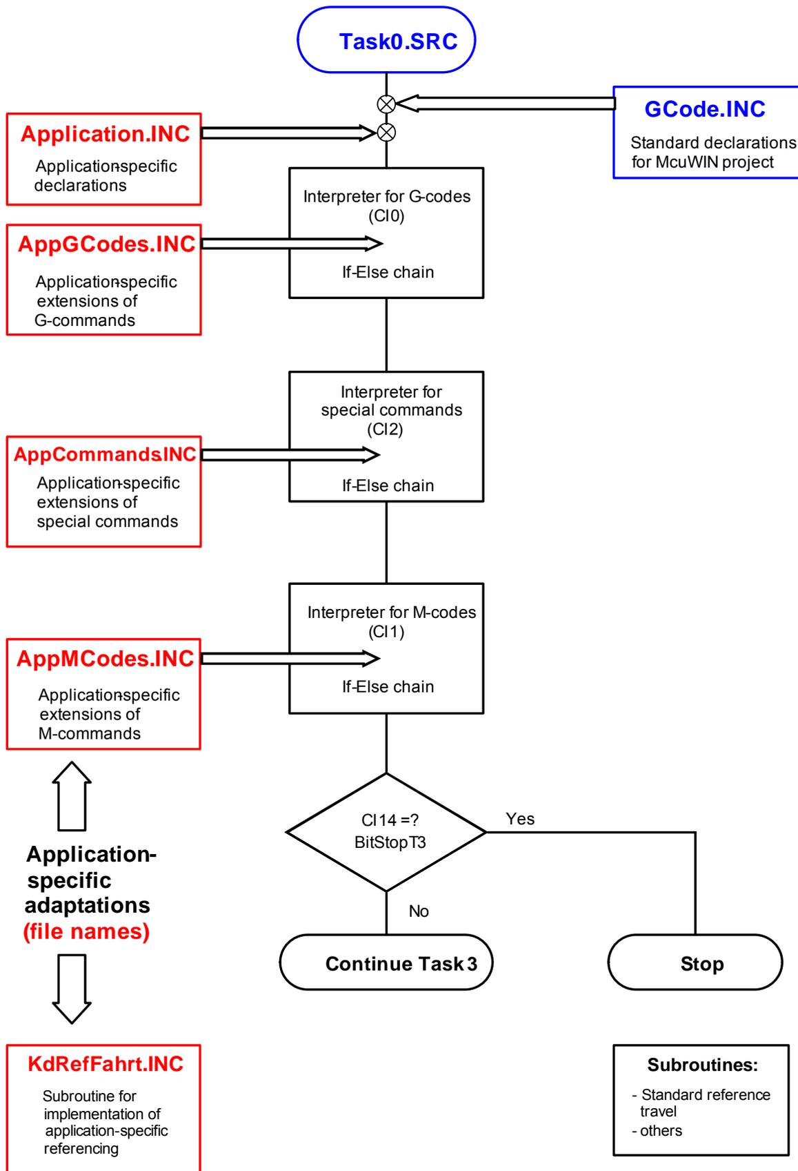
The blocks shown in red on the left-hand side of the flowcharts are the application-specific extensions. These are not replaced in case of updates.
